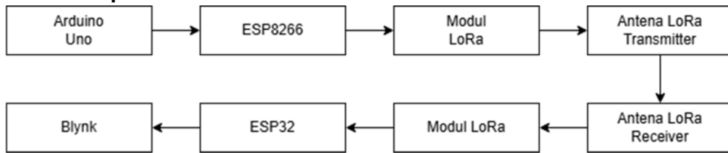
Gambar 14 Diagram Blok Smart Waste System
